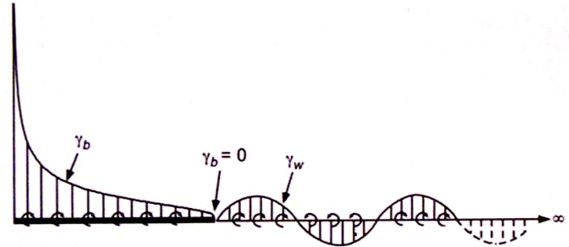
$$C_L = \underbrace{\frac{\pi}{2} \left[ \ddot{h} + \dot{\alpha} - \frac{a}{2} \ddot{\alpha} \right]}_{\text{Added-Mass}} + \underbrace{2\pi \left[ \alpha + \dot{h} + \frac{1}{2} \dot{\alpha} \left( \frac{1}{2} - a \right) \right]}_{\text{Circulatory}} C(k)$$
