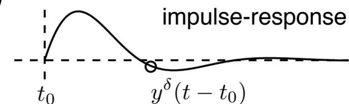
Given a step in angle of attack,  $\dot{\alpha} = \delta(t)$ , the time history of Lift is  $C_L^S(t)$
