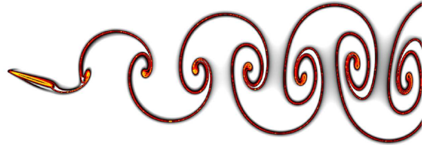
FIG. 13: FTLE field for a pitching flat plate at Re = 100, St = .274 , and T = -15 .
