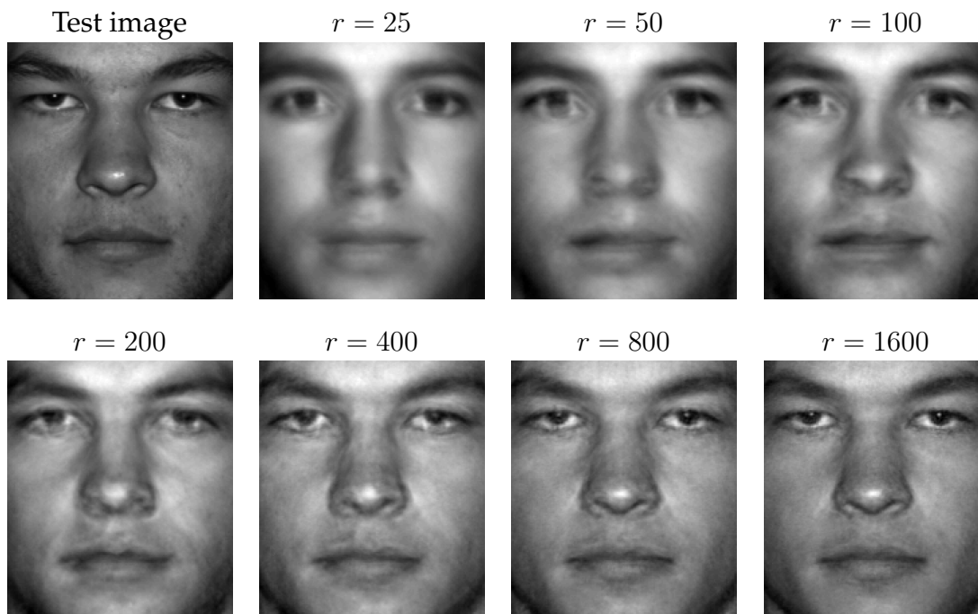
Figure 1.18: Approximate representation of test image using eigenfaces basis of various order r . Test image is not in training set.
