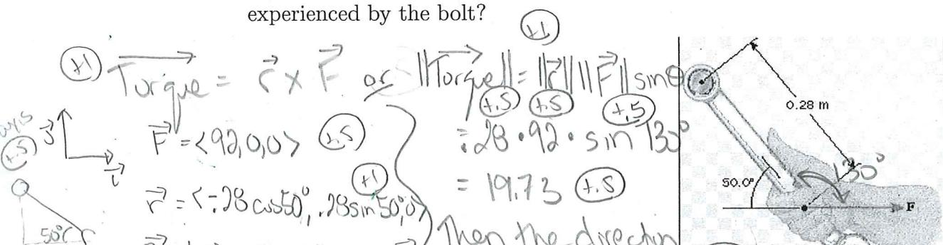
$$\textcircled{1} \quad \text{Torque} = \vec{r} \times \vec{F} \text{ or } \text{Torque} = \| \vec{r} \| \| \vec{F} \| \sin \theta$$
