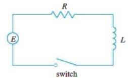
Ohm's Law gives the drop in voltage due to the resistor as RI. The voltage drop due to the inductor **switch** is L(dI/dg). Once of Kirchhoff's laws says that the sum of the voltage drop is equal to the supplied voltage E(t).
