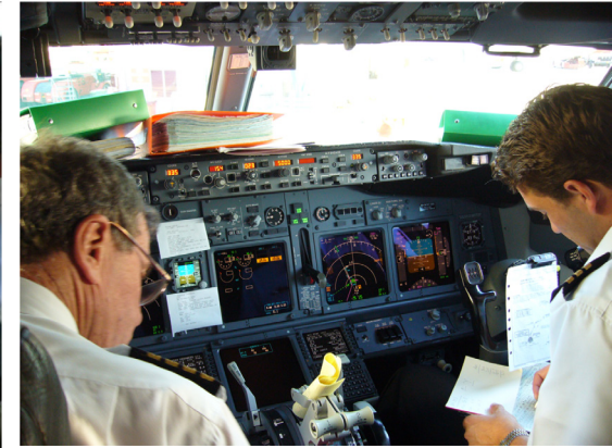
Figure 2. A current glass cockpit with the main flight display suite of large integrated digital displays.
