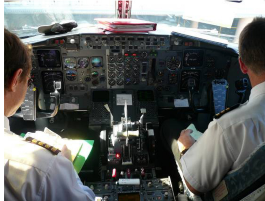
Figure 1. A typical gauge- and dial-based flight deck pre-1984 comprised of an array of analog displays for the different flight data components
