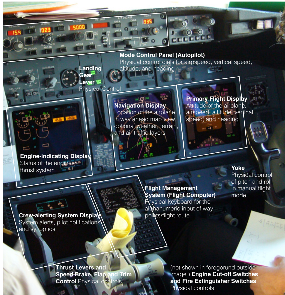
Figure 5: Current pilot display suite in the commercial glass cockpit with call-outs of key instruments and physical controls.
