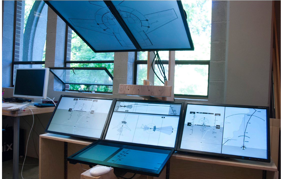
(Above) Figure 26: Full scale flight deck mock-up equipped with six 19" LCD displays for the six-panel video prototype.
