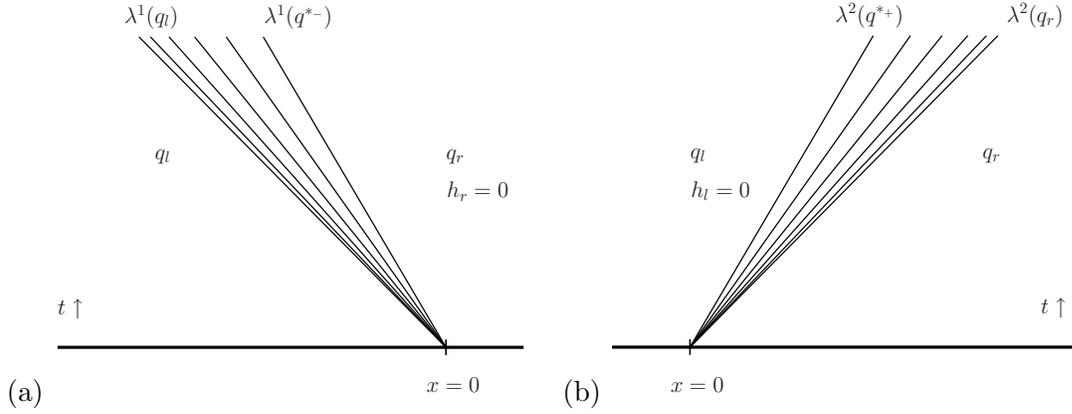
Figure 4.7: The initial dry bed Riemann problems in the  $x-t$  plane. (a) The 1-wave when  $h_r = 0$ . The wet/dry interface moves with speed  $\lambda^1(q^{*-}) = u_l + 2\sqrt{gh_l}$ . (b) The 2-wave when  $h_l = 0$ . The wet/dry interface moves with speed  $\lambda^2(q^{*+}) = u_r - 2\sqrt{gh_r}$ .
