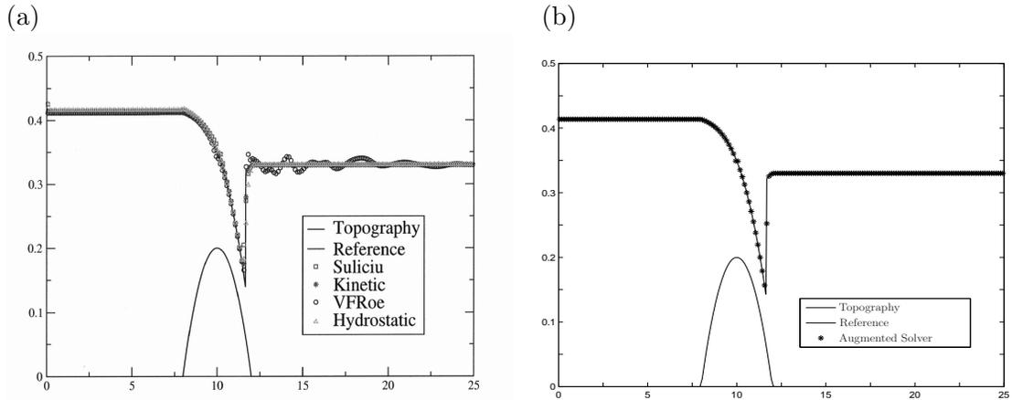
Figure 9.1: Transcritical flow with a shock. The water elevation is shown for the eventual steady state that is reached. (a) Various numerical solutions using methods described in [10] are shown. Figure is borrowed directly from Bouchut [10]. (b) The solution using the augmented approximate solver described in Chapter 6 and the wave propagation methods described in Chapter 3. Both figures show the solution at  $t = 200$ .
