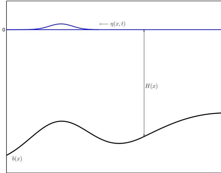
Figure 5.2: Deviation from the physically common steady state: a small perturbation of amplitude  $\eta$  propagates against the background state with depth  $H(x) = -b(x)$ . The figure does not depict a realistic scale, since for a real tsunami  $|\eta| \ll H$ .
