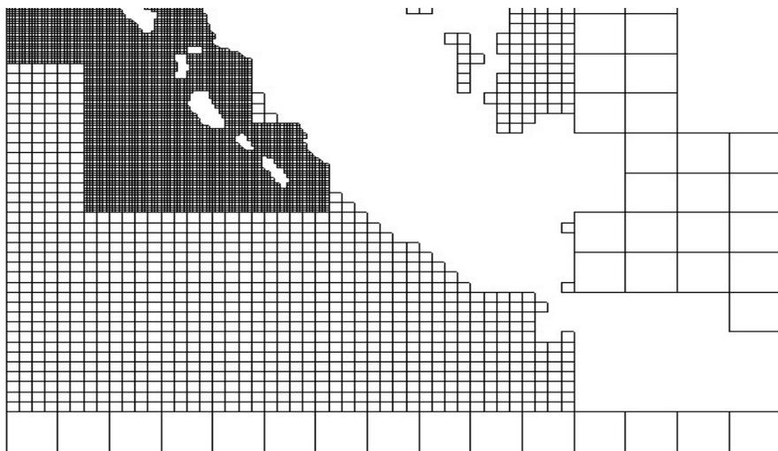
Figure 7.5: Adaptive mesh refinement around a shoreline. The grids are the same set of grids shown in Figure 7.1, covering Sumatra and some surrounding islands. The dry cells are erased to emphasize the shoreline, and show how refinement around the shoreline must necessarily change the overall mass if the true bathymetry is used and the steady state is to be maintained.
