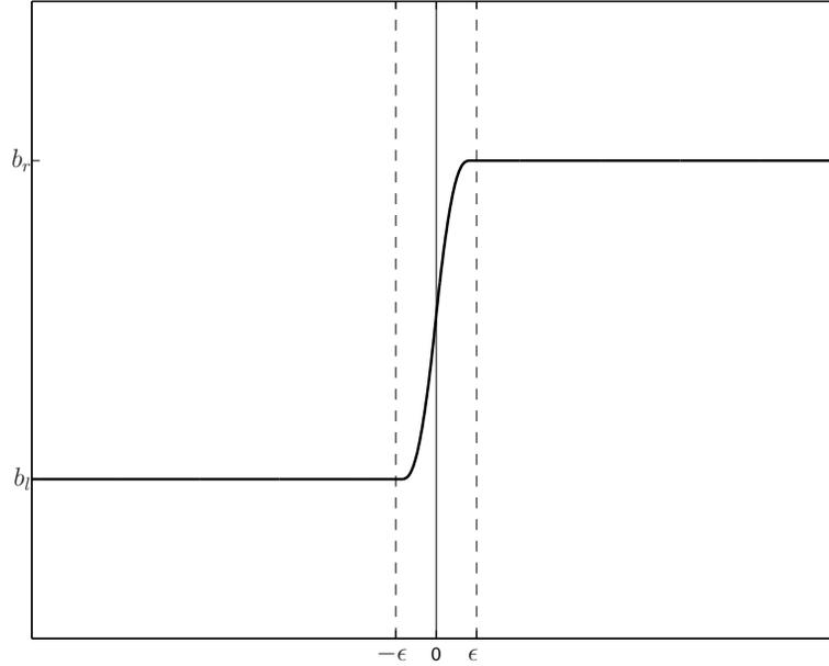
Figure 4.8: A smoothed version of piecewise constant bathymetry. The function shown is  $C^\infty(\mathbb{R})$ , and  $b_x$  has compact support on  $[-\epsilon, \epsilon]$ . Additionally the function is symmetric,  $b(0) = (b_r + b_l)/2$ .
