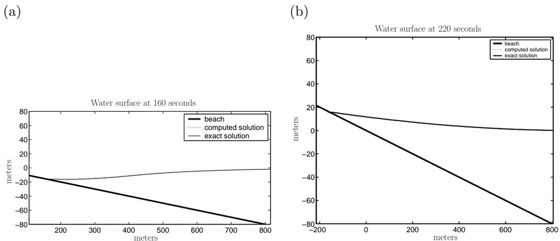
Figure 9.6: Benchmark 1 from the Long Wave Workshop [70]: The surface elevation and beach at two times. (a) Water surface elevation at  $t = 160$  seconds. (b) Water surface elevation at  $t = 220$  seconds.
