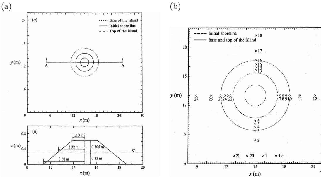
Figure 9.9: Diagram of the conical island wave tank experiment and the location of the gages, from Liu *et al* [72]. (a) Top: top view of the wave tank basin and island. Bottom: vertical view of the circular island on the cross section. (b) Location of the wave gages. The incoming soliton comes from  $y = 0$  from the bottom of the figure. Figures are borrowed directly from [72].
