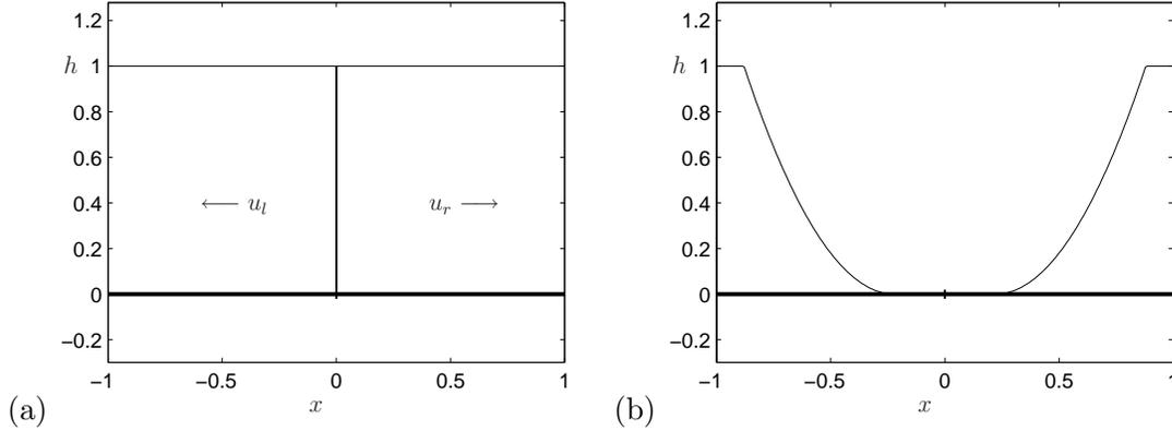
Figure 4.3: An incipient cavitation Riemann problem. (a) The Riemann problem at  $t = 0$ , with  $\Delta u > (\Delta u)_{crit}$ . (b) The Riemann problem at  $t = 3$ . The strong double rarefaction creates an expanding dry middle region.
