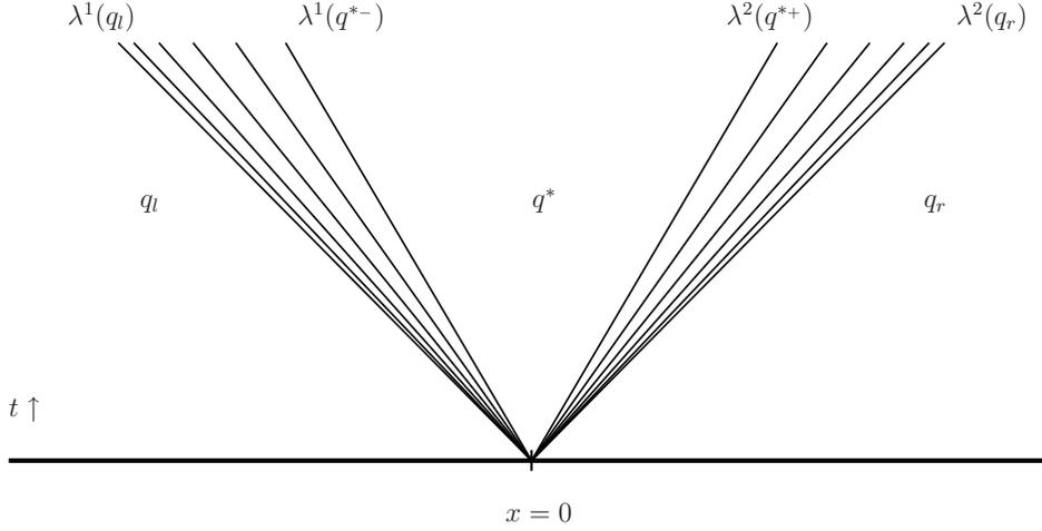
Figure 4.5: The incipient cavitation Riemann problem in the  $x$ - $t$  plane. A strong double rarefaction leads to a dry middle state  $h^* = 0$ . The wet/dry interface on the left moves with speed  $\lambda^1(q^{*-}) = u_l + 2\sqrt{gh_l}$  and the wet/dry interface on the right moves with speed  $\lambda^2(q^{*+}) = u_r - 2\sqrt{gh_r}$ .
