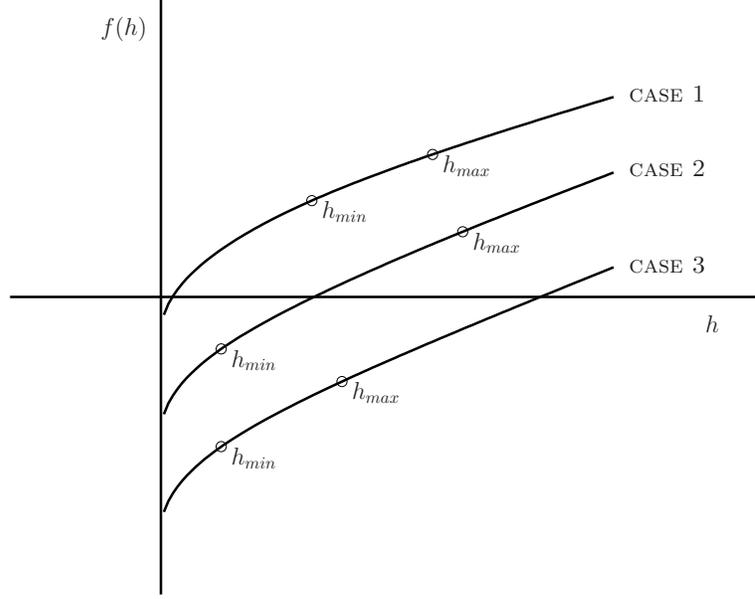
Figure 4.2: Characterization of the Riemann problem for the shallow water equations by function evaluation. The middle state depth  $h^*$  is the root of  $f(h)$ . The graph shows an example of  $f(h)$  for each of the three possible cases in (4.33). Note that  $\Delta u$  shifts the curve for  $f(h)$  up or down. Large values of  $\Delta u$  can therefore ensure CASE 1, or may even eliminate a positive root  $h^*$
