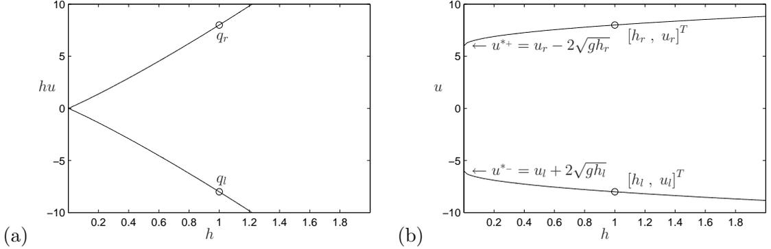
Figure 4.4: Integral curves for the incipient cavitation problem with  $\Delta u > (\Delta u)_{crit}$ . (a) Curves plotted in the  $h$ - $hu$  phase plane. The curves reach the origin  $h = 0$  before intersecting. (b) Curves in the  $h$ - $u$  plane. The  $r^1$  integral curve approaches  $h = 0$  at the point  $u^{*+} = u_r - 2\sqrt{gh_r}$  and the  $r^2$  integral curve approaches  $h = 0$  at  $u^{*-} = u_l + 2\sqrt{gh_l}$ . For the solution shown in these figures  $g = 1$ .
