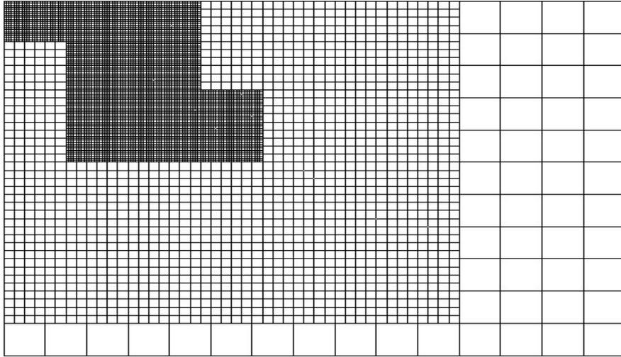
Figure 7.1: Example of adaptive mesh refinement with rectangular Cartesian grids. A portion of the domain is shown with three levels of grids refined by factors of 4. Typically many grids at a given level ( $> 1$ ) may coexist refining important features in the solution with rectangular patches.
