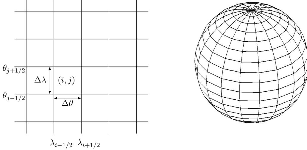
Figure 8.2: Earth-fitted grids: mapping of latitude  $\lambda$  and longitude  $\theta$  coordinates in uniform computational space (left) to a curved grid on the surface of a reference ellipsoid (right). Coordinate Mapping is locally orthogonal.
