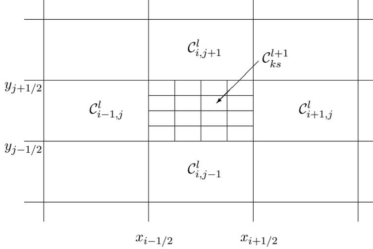
Figure 7.2: Interpolation and averaging between level  $l$  and  $(l+1)$  grids. Using refinement ratios of 4 as an example, the 16 level  $(l+1)$  grid cells within a single level  $l$  cell  $C_{ij}^l$  are shown. Linear interpolation to determine the fine grid cell values, based on (7.4), preserves conservation as can be seen by considering symmetry. Arithmetic averaging of the fine grid cell values to determine the coarse cell value also preserves conservation.
