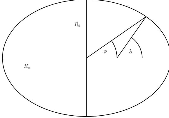
Figure 8.3: Geographic latitude on an oblate ellipse. The cross section of an oblate ellipse with a single equatorial radius  $R_a$  and smaller polar radius  $R_b$  is shown. The geographic latitude  $\lambda$  of a point is the angle between the normal direction and the equatorial plane, not the standard angular coordinate  $\phi$ .
