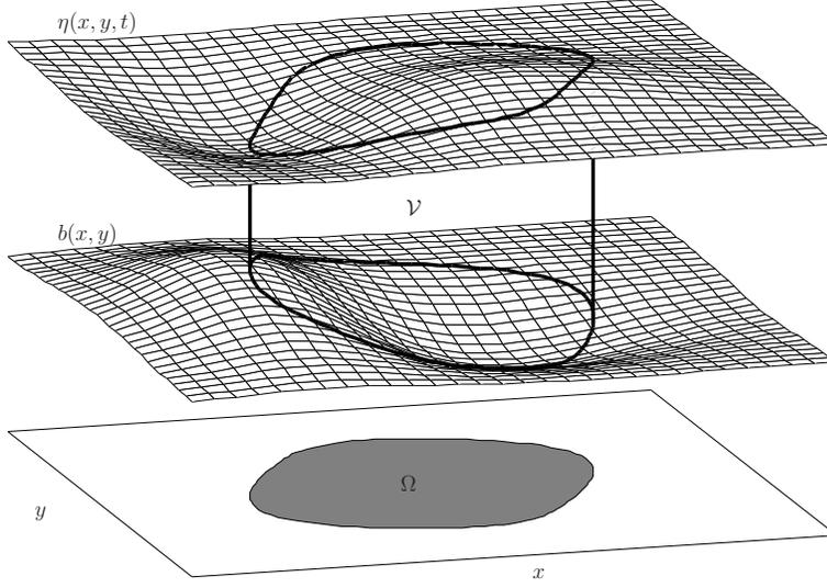
Figure 4.1: Deriving the shallow water equations from conservation principles. The three dimensional control volume  $\mathcal{V}$  and the two dimensional region  $\Omega$  that remains after the vertical dimension is integrated out, are shown. The shallow water equations are a hyperbolic conservation law in the two dimensional  $x$ - $y$  plane.
