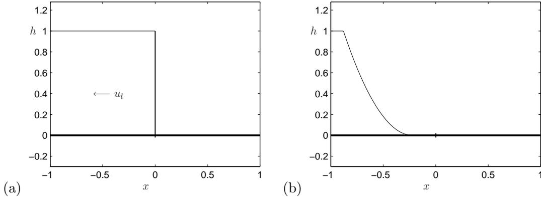
Figure 4.6: An initial dry bed Riemann problem. (a) The Riemann problem initially has a dry state  $h_r = 0$  adjacent to a wet state  $h_l$ . (b) The solution at  $t = 3$  where  $q_l$  is identical to that shown in Figure 4.3. The rarefaction has the same structure as the 1-rarefaction in Figure 4.3.
