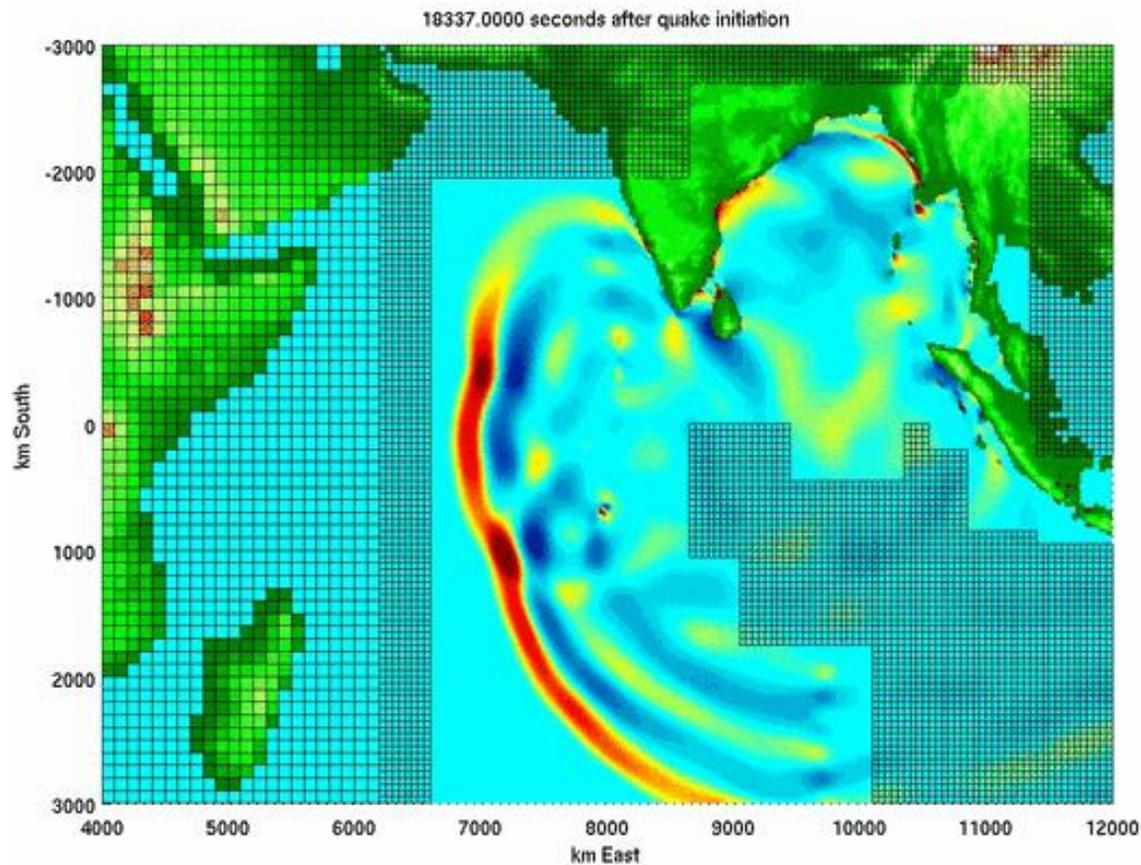
Figure 10.1: Simulation of the Indian Ocean Tsunami showing the entire Indian Ocean on three grid levels. Grid lines are omitted from the finest level.
