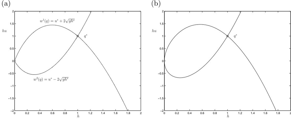
Figure 2.4: (a) Integral curves of the shallow water equations: each curve is tangent to one of the eigenvectors at each point in the phase plane and corresponds to a constant of a Riemann invariant  $w^p(q)$ . (b) Hugoniot loci of the shallow water equations: each curve represents states that can be connected through a shock in the 1<sup>st</sup> or 2<sup>nd</sup> family.
