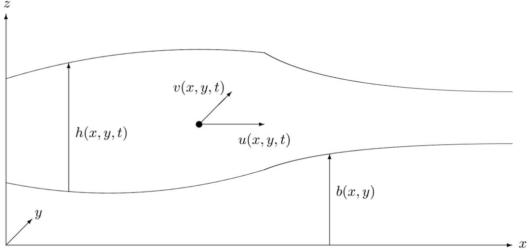
Figure 2.1: Cross section of a free surface flow governed by the shallow water equations (2.1). The fluid depth is  $h(x, y, t)$ , the fluid velocities are  $u(x, y, t)$  and  $v(x, y, t)$ , and  $b(x, y)$  is the bottom elevation. The moving free surface is at  $z = h(x, y, t) + b(x, y)$ .
