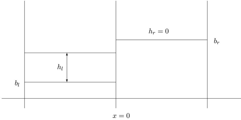
Figure 6.6: A Riemann problem at the shoreline, showing  $h_l + b_l < b_r$ . If this Riemann problem represents the steady state where  $u_l = 0$ , solving it without modification will result in spurious waves from the shoreline.
