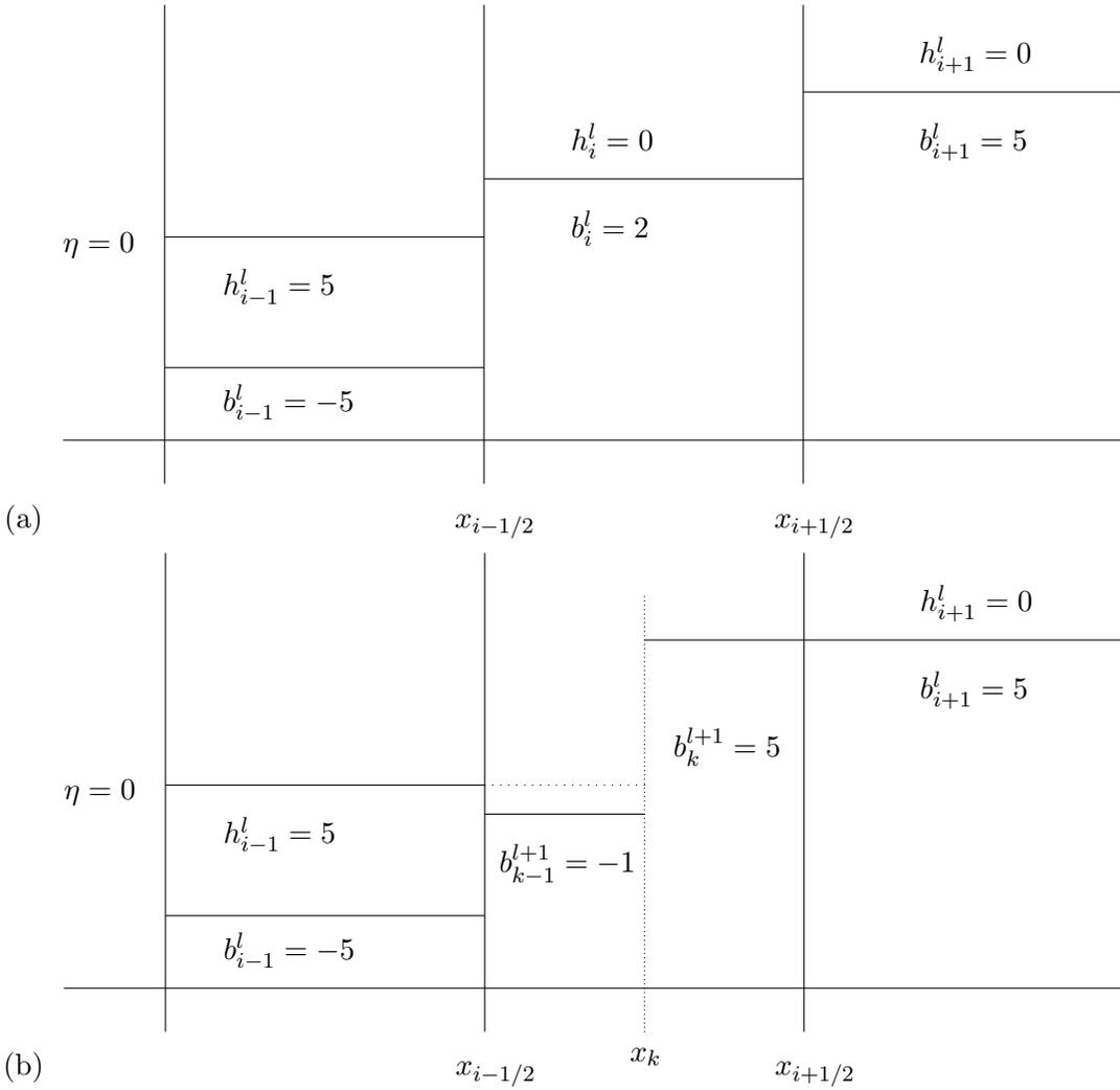
Figure 7.4: Interpolation at the shoreline. (a) Coarse level  $l$  grid at the shoreline where  $h_i^l=0$  and the cell to the left is wet with  $\eta_{i-1}^k = 0$ . This reflects the common steady state problem at the shoreline. (b) Interpolation to fine grid cells within  $[x_{i-1/2}, x_{i+1/2}]$ . Note that to maintain the steady state the surface elevation should be constant across the interface  $x_{i-1/2}$ , implying that  $h_{k-1}^{l+1} = 1$  and  $h_k^{l+1} = 0$ .
