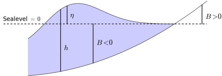
Figure 3: Illustration showing the notation used in the shallow water equations (1).
