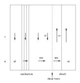
Jump in shear velocity v is advected with velocity  $u_m$ . (Linearly degenerate) Note: Variations in v (y-velocity) in the x-direction do not compress fluid.
