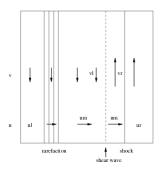
Jump in shear velocity v is advected with velocity  $u_m$ . (Linearly degenerate) Note: Variations in v (y-velocity) in the x-direction do not compress fluid. (Elasticity: restoring force from shear deformation  $\implies$  shear waves.)
