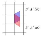
Decompose  $\mathcal{A}^+ \Delta Q_{i-1/2,j}$  into eigenvectors of *B*. Down-going:
