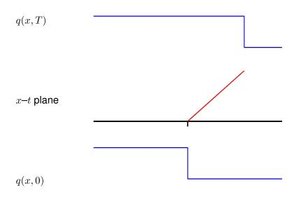
Note: The Riemann solution is not a classical solution of the PDE  $q_t + uq_x = 0$ , since  $q_t$  and  $q_x$  blow up at the discontinuity.
