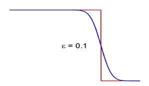
Vanishing Viscosity solution: The Riemann solution q(x,t) is the limit as  $\epsilon \to 0$  of the solution  $q^\epsilon(x,t)$  of the parabolic advection-diffusion equation
