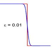
Vanishing Viscosity solution: The Riemann solution q(x,t) is the limit as  $\epsilon \to 0$  of the solution  $q^\epsilon(x,t)$  of the parabolic advection-diffusion equation
