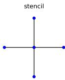
Matrix has block tridiagonal structure:
