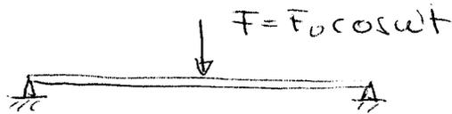
Determine the deflection of the beam when subjected to the shown loading. The beam is at rest at  $t=0$ .
