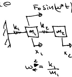
$$\text{where } \Delta(\omega_*) = \begin{vmatrix} k_1 + k_2 - m_1 \omega_*^2 & -k_2 \\ -k_2 & k_2 - m_2 \omega_*^2 \end{vmatrix}$$
