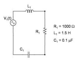
The voltage source is a square wave with period T and amplitude 1.0 V peak-to-peak, i.e.,
