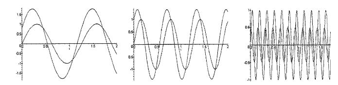
(c) As the input frequency increases (i) the output amplitude decreases, and (ii) the phase shift becomes more negative.
