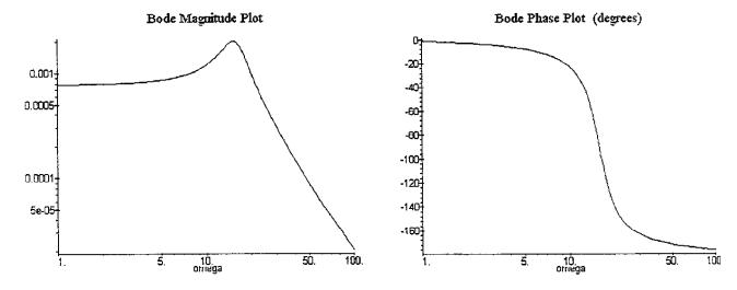
Any noise components with frequencies in the range of approximately 9-30 rad/s will be amplified by the system.
