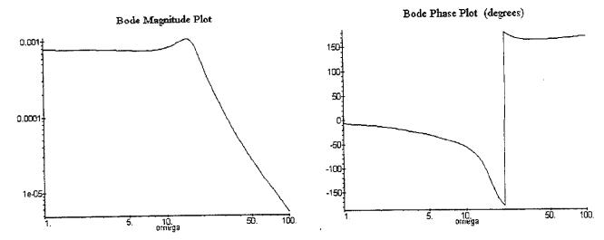
Clearly the last case reduces the effects of the system resonance in the overall response.
