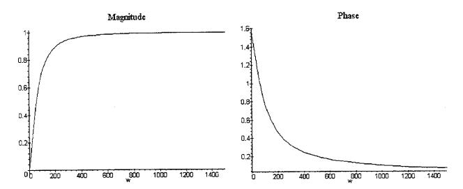
(c) This is a high-pass system begause as the frequency approaches zero  $|H(j\omega)|$  tends to zero.
