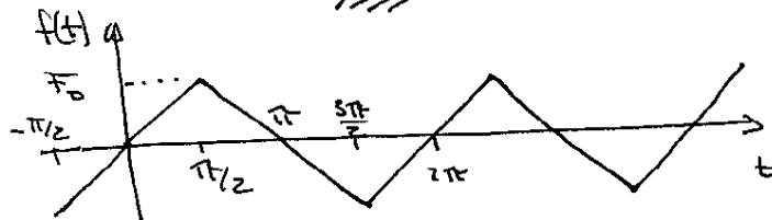
Expand  $f(t)$  using Fourier Series:
