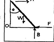
$\theta = 30^{\circ}$ . Apply the static equilibrium conditions to the free body diagram: -F + A = 0, B - W = 0. The moment about the center of mass of the ladder is  $\sum \vec{M}_G = \vec{r}_{B/G} \times (-F\vec{i} + B\vec{j}) + \vec{r}_{A/G} \times A\vec{i}$ ,
