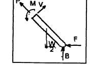
(b) Dynamic case; the reactions: The force F is zero. From the free body diagram, the application of Newton's second law and the equation of angular motion for the dynamic case yields the three equations:
