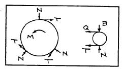
**Problem 7.44** In Problem 7.43, what is the magnitude of the tangential force exerted on the sun gear by each planet gear at their point of contact when the 600 ft-lb couple is applied to the sun gear? Solution:
