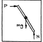
The 18 kg ladder is held in equilibrium in the position shown by the force F. Model Problem 7.77 the ladder as a slender bar and neglect friction. (a) What is the axial force, shear force, and bending moment at the ladder's midpoint? (b) If the force F is suddenly removed, what are the axial force, shear force, and bending moment at the ladder's midpoint at that instant?
