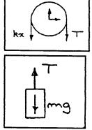
Newton's second law for the mass is  $\sum F = mg - T = ma$ , and the angular equation of motion for the pulley is  $\sum M = RT - Rkx = I\alpha = I\left(\frac{a}{R}\right)$ . Eliminating T, we obtain  $a = \frac{mg - kx}{m + I/R^2}$ . Applying the chain
