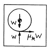
**Problem 7.41** A soccer player kicks the ball to a teammate 20 ft away. The ball leaves his foot moving parallel to the ground at 20 ft/s with no initial angular velocity. The coefficient of kinetic friction between the ball and the grass is  $\mu_k = 0.4$ . How long does it take the ball to reach his teammate? (The ball is 28 in. in circumference and weighs 14 oz. Estimate its moment of inertia by using the equation for a thin spherical shell:  $I = \frac{2}{3}mR^2$ .)
