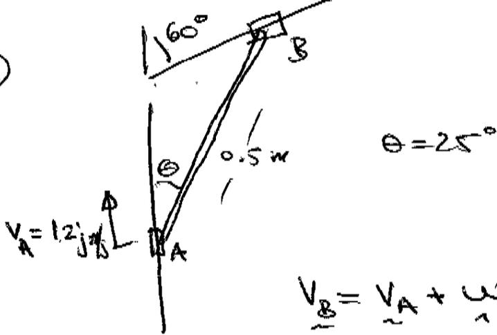
$$\underline{V}_B = \underline{V}_A + \underline{\omega}_{AB} \times \underline{r}_{B/A}$$
