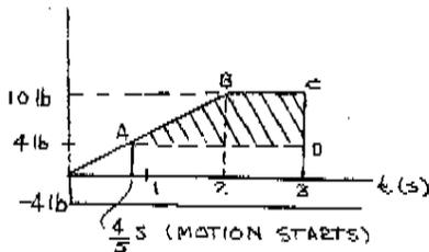
$$AREA_{ABCD} = \text{MAX IMPULSE} = \frac{1}{2}(6 \text{ lb})\left(\frac{6}{5} \text{ s}\right) + (6 \text{ lb})(1 \text{ s})$$
