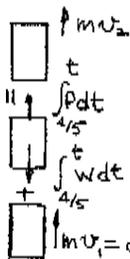
$$m a_1 + \int_{4/5}^t P dt - \int_{4/5}^t W dt = m v_2$$
