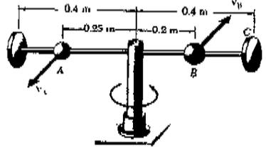
(a) WHEN THE PIN HOLDING BALL B IS REMOVED, THERE ARE THEN NO HORIZONTAL FORCES ACTING ON THE BALL. THEREFORE, AT  $t=0$ ,  $F_r = 0$  AND  $F_\theta = 0$
