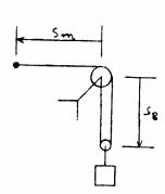
14-59. The 50-lb load is hoisted by the pulley system and motor M. If the motor exerts a constant force of 30 lb on the cable, determine the power that must be supplied to the motor if the load has been hoisted s = 10 ft starting from rest. The motor has an efficiency of  $\epsilon = 0.76$ .
