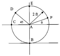
Create two coordinate systems. One fixed to the ground at B and one fixed to the disk (but not rotating) at A.
