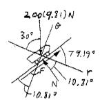
\*13-100. Using a forked rod, a smooth cylinder C having a mass of 0.5 kg is forced to move along the vertical slotted path  $r = (0.5\theta)$  m, where  $\theta$  is in radians. If the angular position of the arm is  $\theta = (0.5t^2)$  rad, where t is in seconds, determine the force of the rod on the cylinder and the normal force of the slot on the cylinder at the instant t = 2 s. The cylinder is in contact with only one edge of the rod and slot at any instant.
