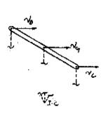
\*18-16. The 4-kg slender rod is subjected to the force and couple moment. When it is in the position shown it has an angular velocity  $\omega_1 = 6 \text{ rad/s}$ . Determine its angular velocity at the instant it has rotated downward 90°. The force is always applied perpendicular to the axis of the rod. Motion occurs in the vertical plane.
