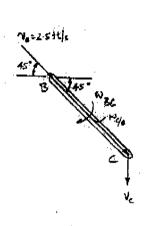
16-95. If the collar at C is moving downward to the left at  $v_C = 8$  m/s, determine the angular velocity of link AB at the instant shown.
