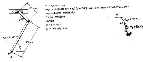
16-55. Determine the velocity of the slider block at C at the instant  $\theta = 45^{\circ}$ , if link AB is rotating at 4 rad/s.
