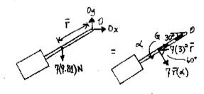
\*17-72. Determine the angular acceleration of the 25-kg diving board and the horizontal and vertical components of reaction at the pin A the instant the man jumps off. Assume that the board is uniform and rigid, and that at the instant he jumps off the spring is compressed a maximum amount of 200 mm,  $\omega = 0$ , and the board is horizontal. Take k = 7 kN/m.
