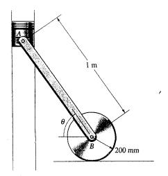
The 2-kg slender bar starts from rest in the vertical position and falls, striking the smooth surface at P. The coefficient of restitution of the impact is e = 0.5. When the bar rebounds, through what angle relative to the horizontal will it rotate?
