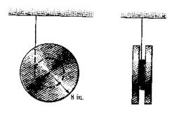
The 100-kg cylindrical disk is at rest when the force F is applied to a cord wrapped around it. The static and kinetic coefficients of friction between the disk and the surface equal 0.2. Determine the angular acceleration of the disk if (a) F = 500 N; (b) F = 1000 N.
