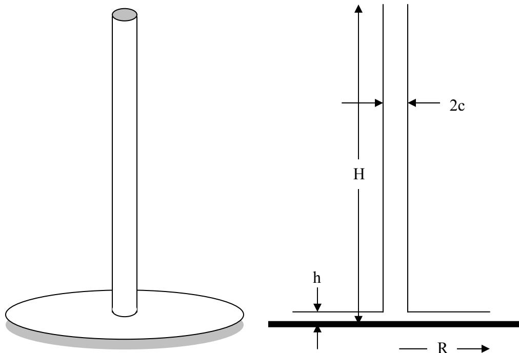
**Figure 1.** Sketch of the solar chimney, with some relevant dimensions
