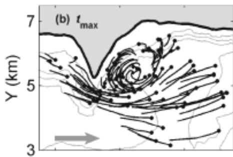
**Figure:** surface Lagrangian drifter tracks during tidal flow past Three Tree Point in Puget Sound, during maximum flood current. The location of each drifter is shown with a dot, and the last hour of its track is shown with a line. The gray region at the top is land. The Point is about 1 km in scale. A large “tidal headland eddy” with positive vertical vorticity is evident to the right of the Point.
