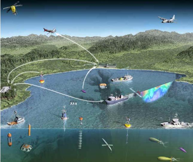
**Figure 6:** Schematic diagram showing the synergistic integration of in situ and remote sensing sensors in Monterey Bay.
