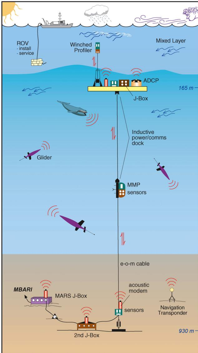
**Figure 1: Moored Sensor Network with Seagliderns planned for the MARS Observatory in Monterey Bay.**
