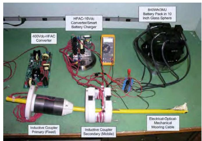
Fig. 6. The inductive power system (IPS) components.
