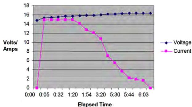
Fig. 8. Plot of the battery voltage and current during charging, measured at the battery.
