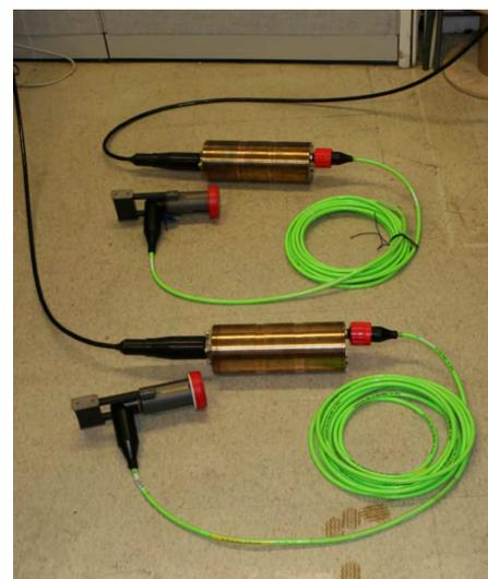
Fig. 3. ROV-mateable connectors and the electro-optical converters (in beryllium copper pressure cases) attached to each end of the (black) seafloor cable.
