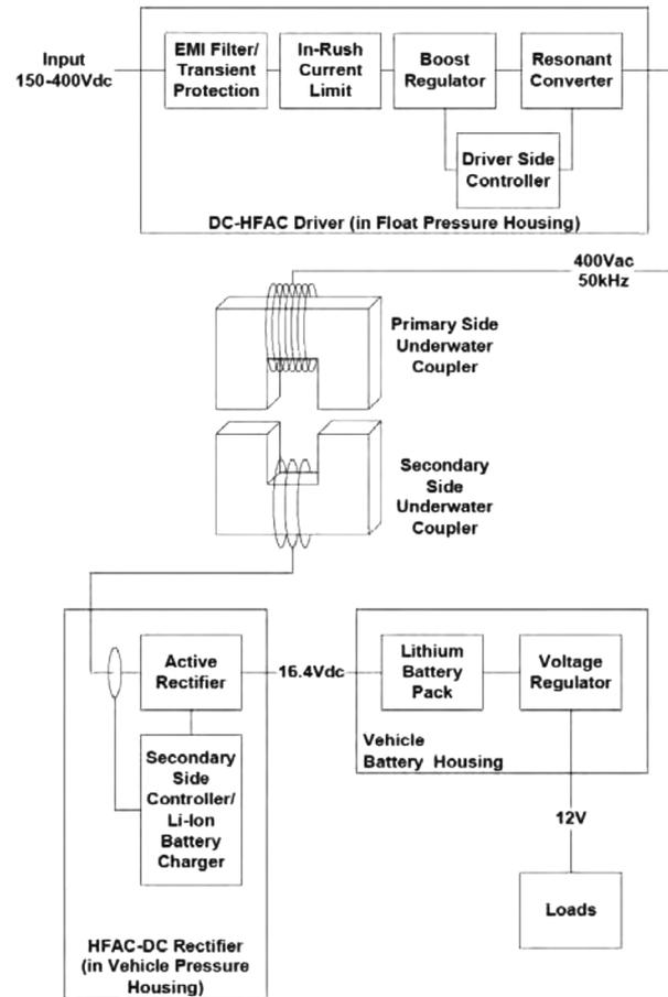
Fig. 5. Inductive power system block diagram. A series resonant converter drives a constant frequency square wave voltage across the inductive coupler that is rectified and regulated on the secondary side.
