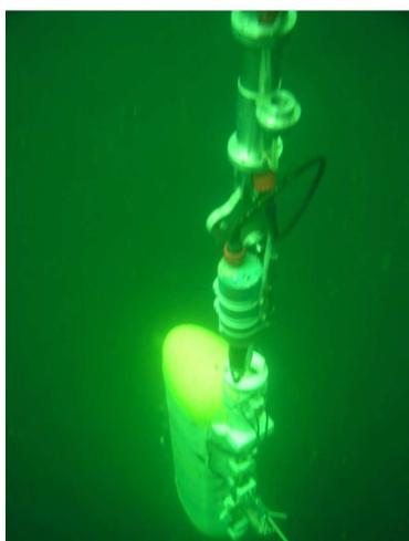
Fig. 7. (top) Deploying the MMP. The inductive power system primary is at the very top on the mooring cable, the secondary is on top of the profiler. The acoustic current meter has the four arms in the middle. The CTD sensors are wrapped in antifouling copper tape. (bottom) The MMP on the mooring in Puget Sound in the docking position. One electro-optical converter is above the dock followed by a D-plate and the electro-mechanical swivel.
