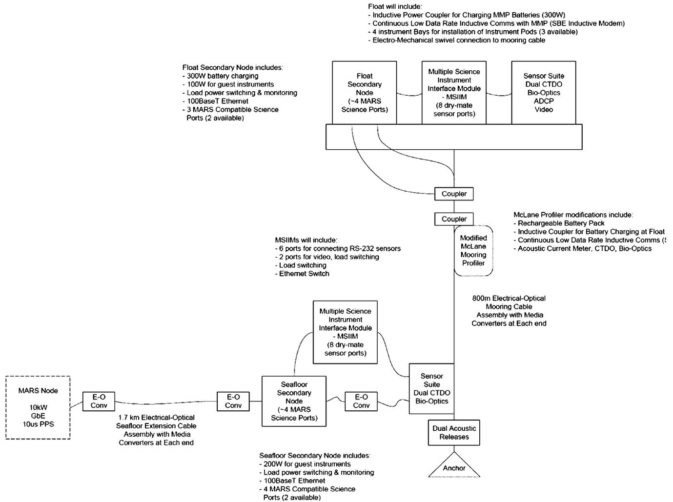
Fig. 2. Mooring system block diagram.
