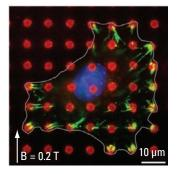
An immunofluorescence micrograph shows focal adhesions (green), microposts (red), and cell nucleus (blue) after force actuation. The direction and magnitude of the magnetic field are indicated. (Adapted with permission. Copyright 2007 National Academy of Sciences, U.S.A.)
