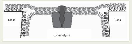
Schematic illustration of the suspended bilayer- $\alpha$ -hemolysin system at the GNP orifice.
