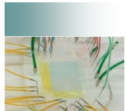
Microfluidics screening device in Dr. Khademhosseini's BiOMEMS research laboratory.
