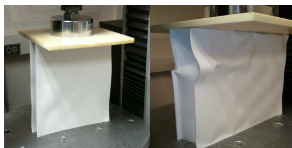
Design of load-bearing panels from flat microcellular PET sheet. Prototype sandwich panel schematic (L) and before (M) and after (R) testing (Sponsor: MicroGREEN Inc., 2012).
