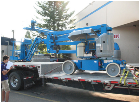
A Genie lift ready to be shipped. Students attached accelerometers to the lift to characterize vibrations and recommended ways to reduce the damage to the lift during transport.
