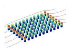
**IMAGE:**This is a simulation of the posts that support the heart cells. Light blue represents 1 nanometer of deflection, while dark red means the post is deflected by 2.5 nanometers....
