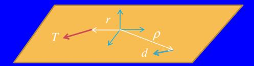
• Green's tensor  $g_{ij}$  gives displacement in i-direction at location  $\rho$  due to concentrated force T at location r acting in j-direction
