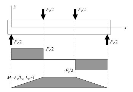
Figure 4 Free Body, Shear Force and Bending Moment Diagrams for Four-Point Flexure Loading
