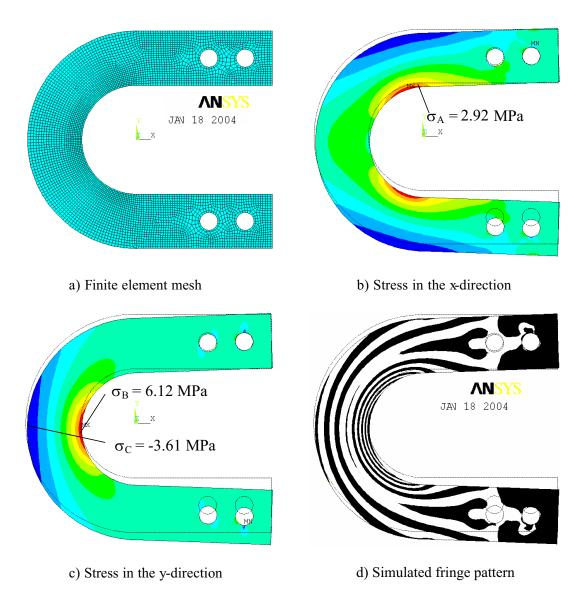
Figure 5 Finite Element Analysis Solution to the Curved Beam Bending Problem
