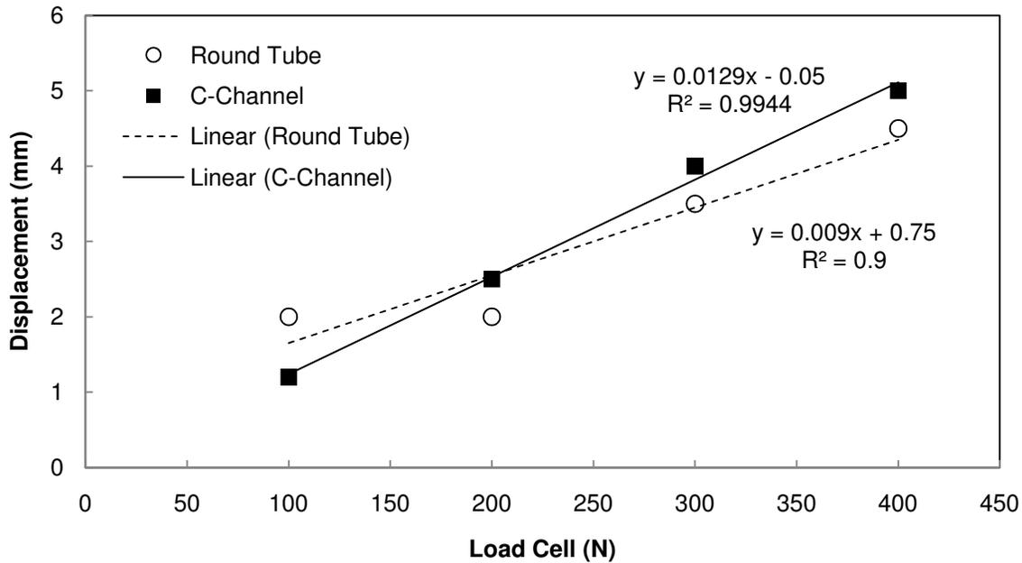
**Figure 2.** Displacement vs. load for each beam design. (Right-click and select “Edit Data” to change values)
