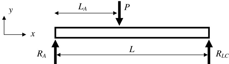
**Figure B.1** Free-body diagram of 3-pt loaded beam.
