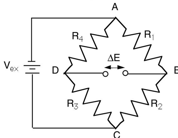
FIGURE 2 - Schematic Diagram of a Wheatstone Bridge
