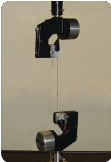
▲ Cord and yarn grips are a unique solution for testing thin wire specimens in tension. The design of the grip prevents jaw breaks that commonly can occur with side acting grips.
