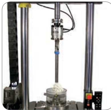
▲ Instron 8874 testing system, and combined temperature controller and recirculation unit, provide a platform for specialized test fixtures to satisfy ASTM standard requirements.
