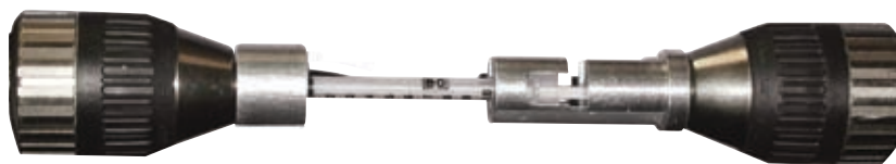
▲ 55MT MicroTorsion system for torsion testing conical lock fittings with luer taper for syringes.
