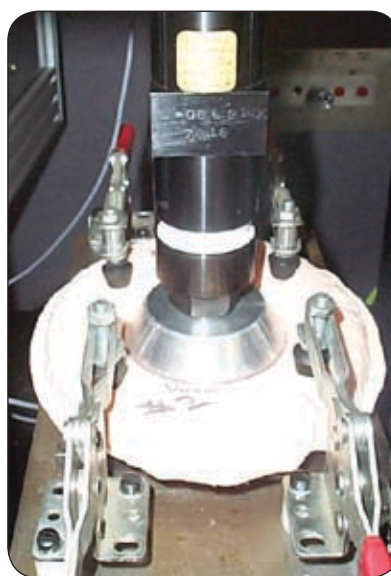
▲ The impact resistance of a hip protector is evaluated using a Dynatup 9250HV impact testing system.
