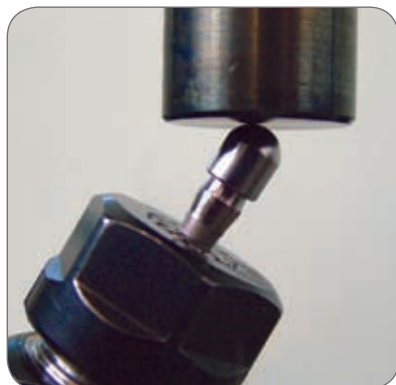
An endosseous implant undergoes compression-bending fatigue.
