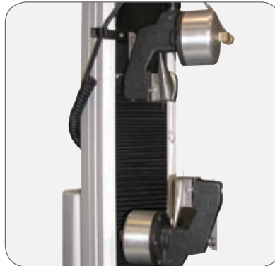
◀ A 3345 universal testing system, configured with pneumatic cord and yarn grips, is used to perform a knot-pull test on suture material.
