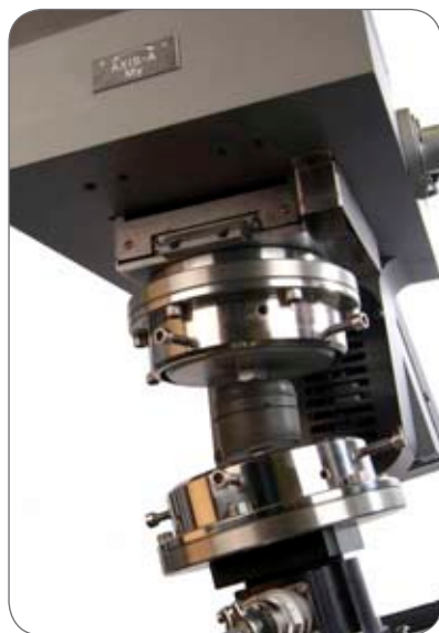
▲ Instron's Spine testing system can apply loads and motions in all six degrees-of-freedom.
