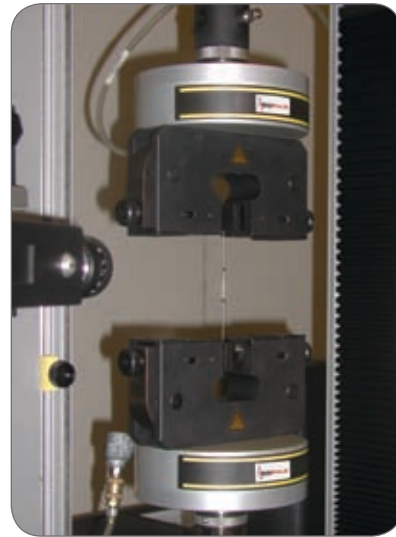
▲ A 5569 universal testing system, 5 kN pneumatic side action grips with serrated faces and a video extensometer are ideal for testing stainless steel tubing in tension with high precision strain measurement.
