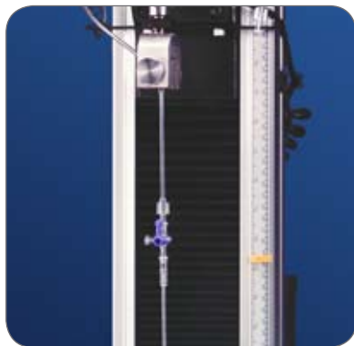
▲ A 5545 universal testing system configured with side action screw grips and serrated faces is used to compare the strength of a fitting with the ultimate strength of the tubing material.
