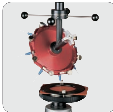
▲ The BioPuls multineedle test fixture (upper) and rotational membrane holder (lower) increase the rate of testing on up to eight needles at multiple penetration points.
