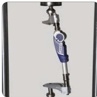
▲ A 3R80 prosthetic knee joint undergoes a structural strength test according to ISO 10328 condition II.
