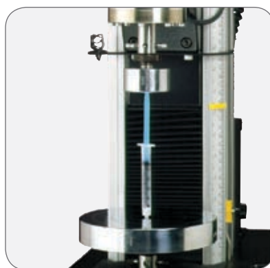
▲ A 5544 universal testing system with standard compression platens can be used to evaluate breakout and sustaining forces required to move the needle plunger.
