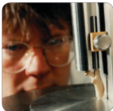
▲ Fixture applies shear loading to the femoral head of a rat femur.
