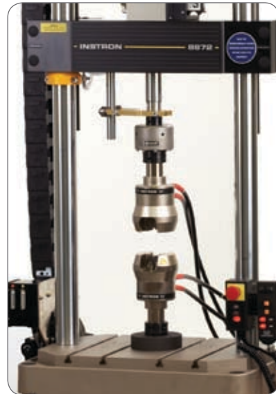
▲ Instron's 8870 range of servohydraulic test systems can perform by static and dynamic testing .
