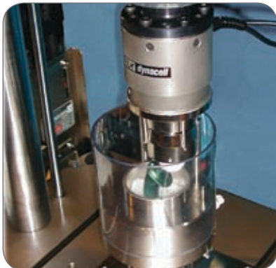
▲ BioPuls femoral fatigue fixture using patented Dynacell™ load cell technology.
