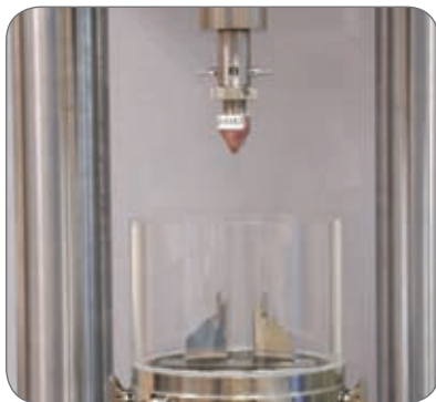
▲ Micro three-point bend fixture with saline tank.
