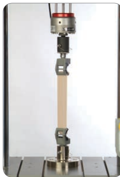
▲ Elastomeric grips are used to evaluate the strength of bandages in tension.
