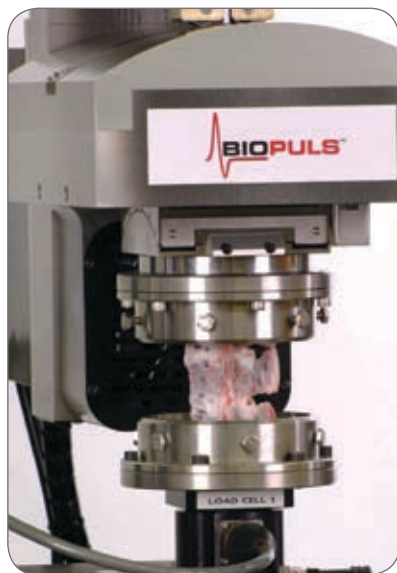
▲ An Instron second generation BioPuls six-axis modular spine testing system.
