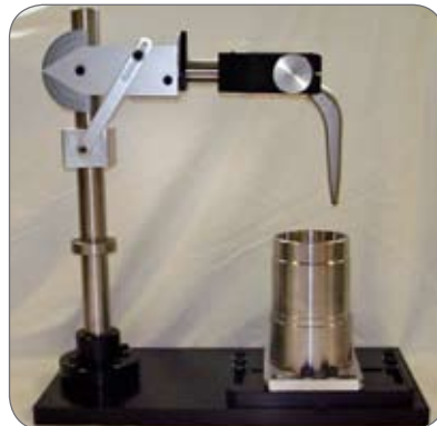
▲ The embedding fixture ensures correct implant alignment for the test.
