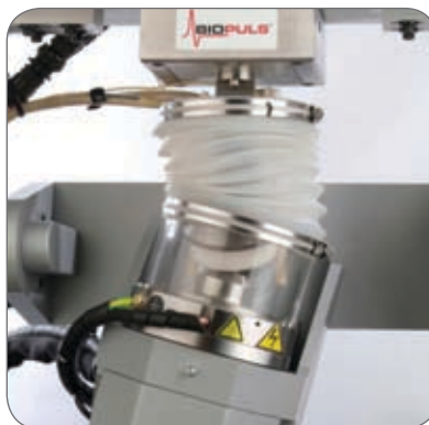
▲ BioPuls ISO hip simulator. The wear test station generates loads and motions within the femoral head.
