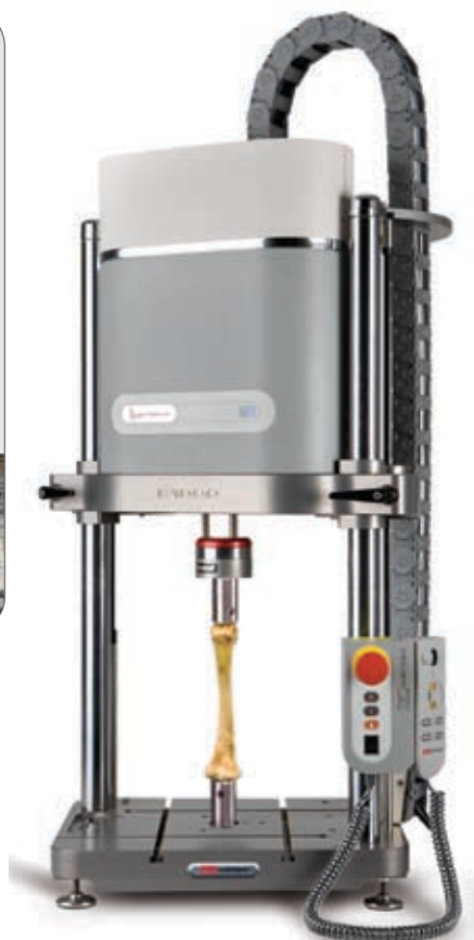
▲ An ElectroPuls® E1000 test instrument performs fatigue testing on a whole bone.
