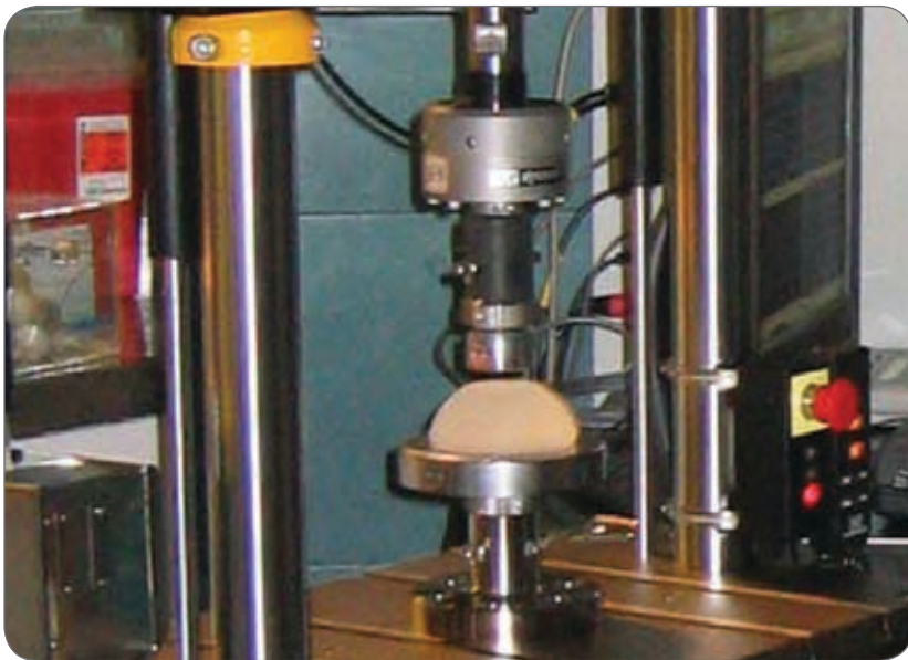
▲ An 8872 fatigue testing system with compression platens evaluates the fatigue properties of a breast implant.
