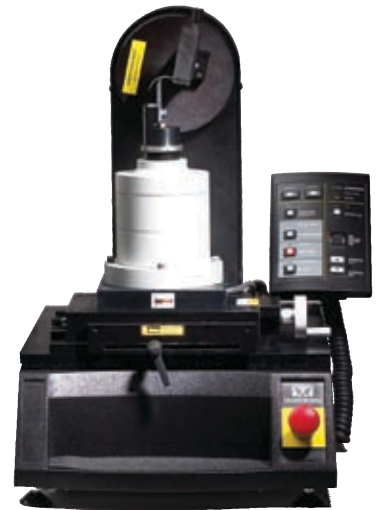
▲ The BioPuls™ curved needle tester is used to ensure that the needle is sharp enough to puncture tissue and strong enough to retain its shape during use.
