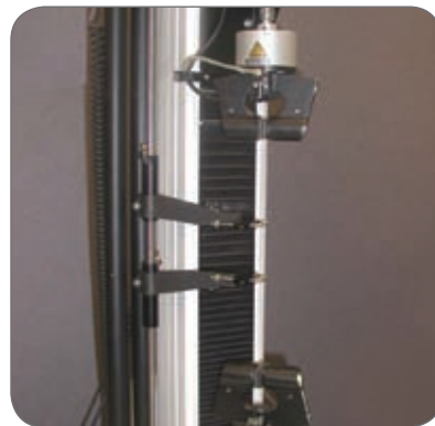
▲ Tensile strength, strain at break and elastic modulus measurements are acquired for thin-wall tubing specimens using a 3345 universal testing system, pneumatic side action grips and a long travel extensometer.
