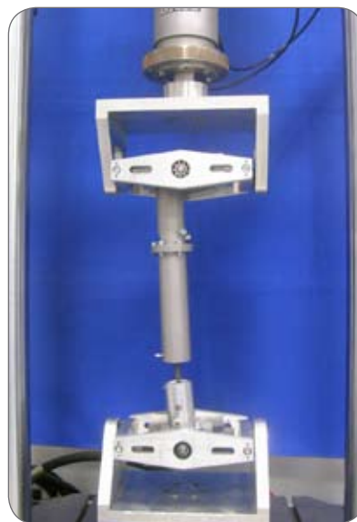
▲ An 8874 axial-torsional servo hydraulic system is used to perform a fatigue test on a femoral nail.
