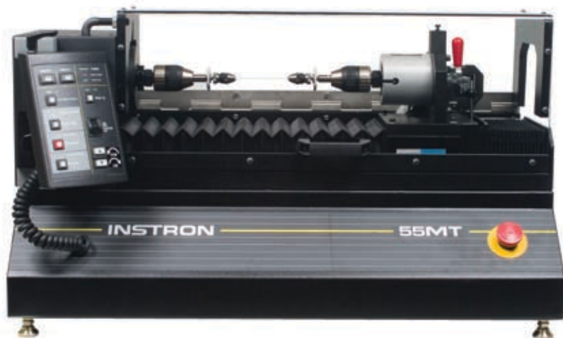
▲ 55MT MicroTorsion system with micro grip chucks for multi-turn torsion testing of surgical tubing.
