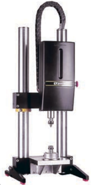
▲ The MicroTester is extremely versatile for a variety of low-force tissue tests in both vertical and horizontal configurations.
