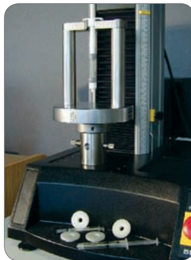
▲ The fixture shown above is used to measure the ejection forces of fluids from the barrel of a syringe. The fixture uses plastic inserts to hold a variety of different syringe sizes and diameters.
