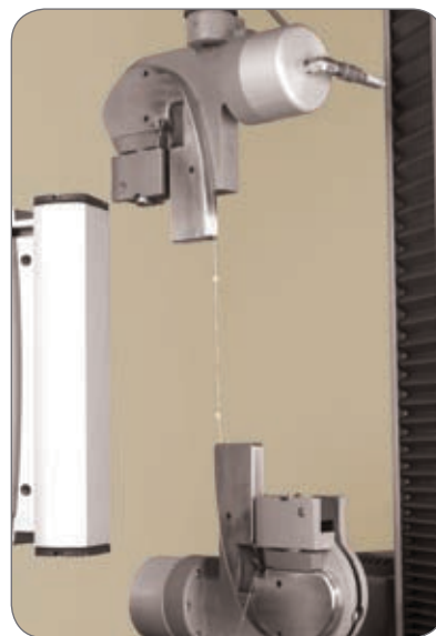
▲ Pneumatic cord and yarn grips, and the video extensometer are successfully able to test the ultimate strength of nitinol wire without premature failure of the specimen as a result of gripping or measuring strain.
