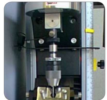
▲ A single straight needle fixture (upper) and variable angle membrane holder (lower) are often used in research and development processes for characterizing needle sharpness.
