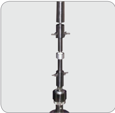
Fixtures enable tensile adhesion strength of dental materials to be evaluated.
