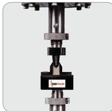
Micro three-point bend fixture for flexural tests.
