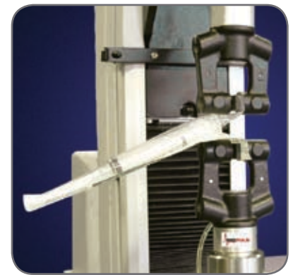
A 3342 universal testing system with 250 N capacity pneumatic side action grips and line contact faces is used to grip disposable syringe packaging in a T-peel test. Such tests allow quality personnel to investigate the seal strength of their packaging methods and to ensure the sterility of the devices after delivery.
