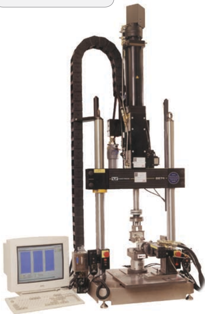
▲ An 8874 testing system with anterior-posterior actuator studying laxity and tribology.
