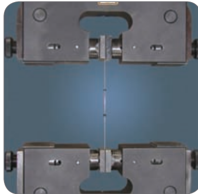
▶ A close-up of the stainless steel tubing specimen shown above. The gripped ends of the tubing are filled with inserts to maintain the tubing geometry and prevent jaw breaks. The 25.4 mm (1 in) gauge length is marked with 2 mm wide black tape wrapped around the diameter of the specimen.
