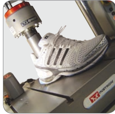
▲ ElectroPuls E3000 electrodynamic test instrument performing impulse tests on training shoe.
