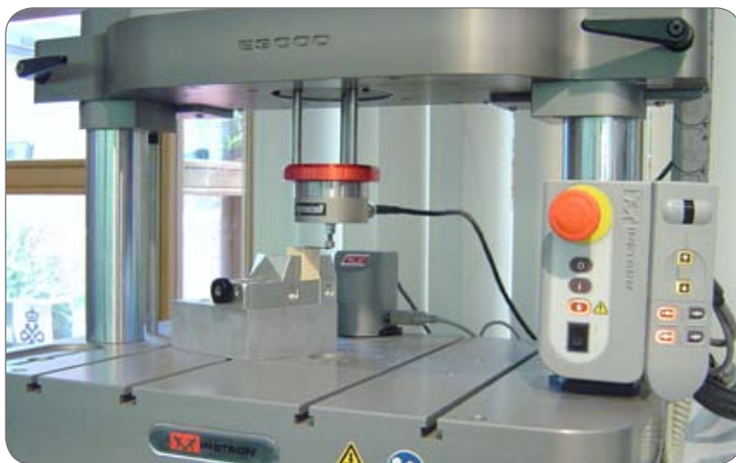
▲ A craniomaxillofacial implant is tested on an ElectroPuls® E3000 system at 20 Hz using a low-force Dynacell load cell.
