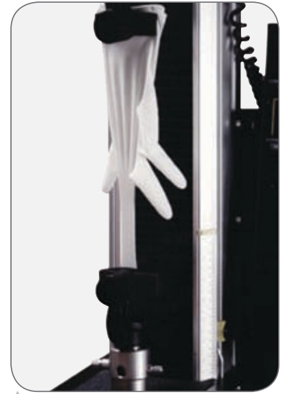
A 5544 universal testing system configured with side action screw grips and rubber-coated faces can be used for evaluating the tensile strength of medical gloves.
