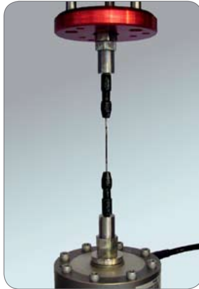
▲ ElectroPuls® E1000 performs a high-frequency fatigue test on 300 micron-diameter wire using lightweight collet grips.
