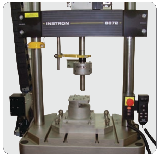
▲ A 8872 servohydraulic fatigue system with BioPuls tibial tray fixture.
