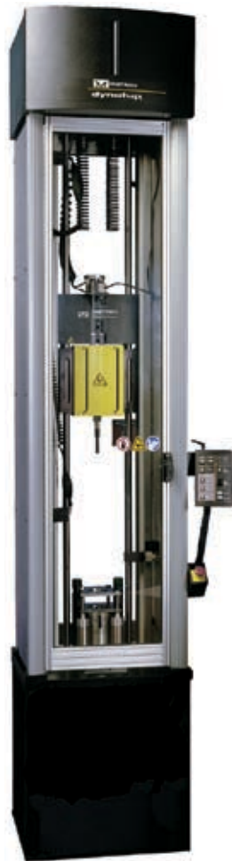
▲ The Dynatup 9250HV drop tower is used to evaluate the strength of the implant under impact.
