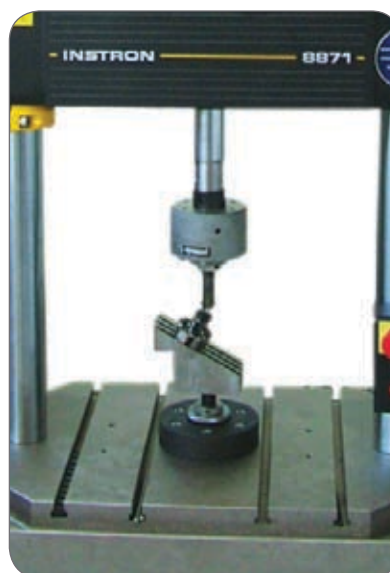
The dental implant fatigue fixture can be fitted to a 8870 servo hydraulic system or an ElectroPuls® Electrodynamic system.
