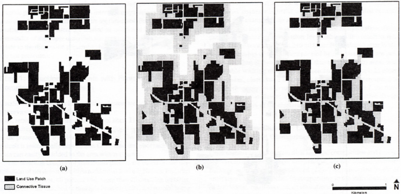
FIGURE 3 Simplified steps in delineation of land use clusters: (a) land use patches; (b) extended patch boundaries; (c) spatial clusters of patches.
