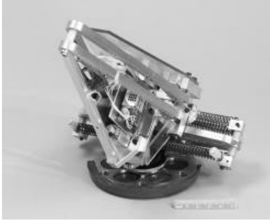
Figure 5: Photo of 2 nd Generation hopper in compressed state.
