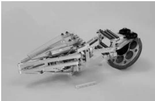
Figure 6: (a) Photo of 2 nd generation thrust leg uncompressed.
