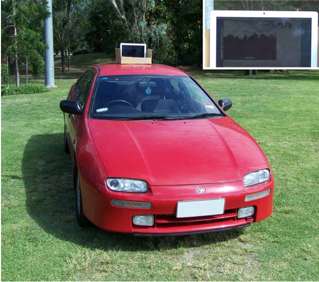
Fig. 5. Apple Macbook with built-in iSight video camera (inset) mounted on the test vehicle. This camera was the sole source of sensory information for the mapping system. The laptop was mounted on the roof of the car in a forward facing, zero pitch position.
