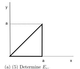
A waveguide is constructed so that the cross section of the guide form a triangle with sides of length a, a and  $\sqrt{2}a$  as in the figure. The walls are perfect conductors and  $\epsilon = \epsilon_0$ ,  $\mu = \mu_0$  inside the guide. Consider **only** TE electromagnetic waves, and  $B_z$  of the form  $B_z(x, y, z, t) = f(x, y)e^{ikz-i\omega t}$ .
