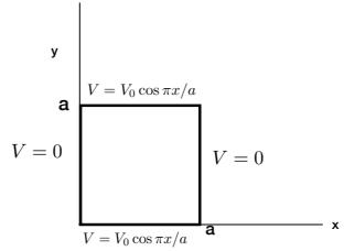
(a) (6) Explain why the function  $f_n(x, y) \equiv \sin \frac{n\pi x}{a} \cosh[\frac{n\pi}{a}(y - a/2)]$ , where  $n$  is an integer  $\geq 1$  is a solution of Laplace's equation.
