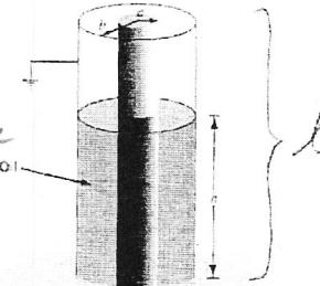
$$\text{Capacitance above oil } C_1 = \frac{\lambda(l-h)}{4\pi} = \frac{2\pi \epsilon_0}{\ln(b/a)} (l-h)$$
