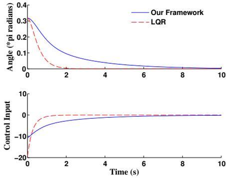
Fig. 2. Pendulum: LQR vs Our Framework
