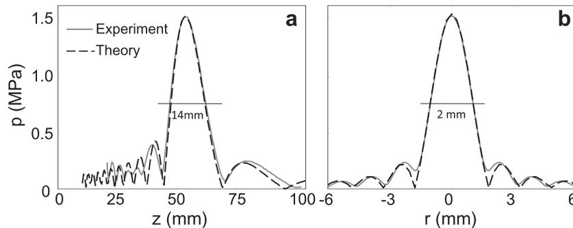
Fig. 2. Acoustic pressure field of the transducer used for ultrasound-induced hyperthermia: (a) axial, (b) transverse. *Solid lines* represent measurements, and *dashed lines* represent theoretical predictions based on the Rayleigh integral.
