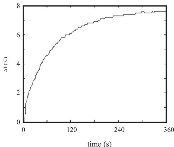
Fig. 5. Temperature elevation of OptiMEM in the sample holder caused by thermal conduction from the glycerol. Ultrasound conditions:  $p = 1.6$  MPa,  $f = 1.1$  MHz, 500 cycles, 45% duty cycle.
