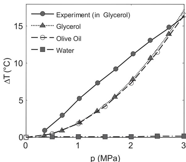
Fig. 4. Predictions of temperature elevation as a function of pressure at focus for different media and comparison with measured values in glycerol. Ultrasound conditions: 1.1 MHz, 500 cycles, 45% duty cycle, 20-s duration.
