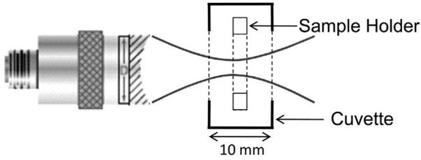
Fig. 1. Ultrasound exposure setup with focused transducer and double compartment, the outer filled with glycerol and the inner filled with cell culture medium (OptiMEM). *Dotted lines* represent Mylar acoustic windows on the cuvette (outer compartment with dimensions  $10 \times 10 \times 30$  mm) and sample holder (3-mm-diameter inner compartment) walls. The sample holder is placed at the focus of the transducer.
