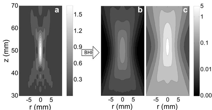
Fig. 3. (a) Contour plot of the axial pressure distribution [plane ( $r = 0, z$ )]. (b, c) Predicted temperature elevation after 20 s of ultrasound exposure in water (b) and glycerol (c).
