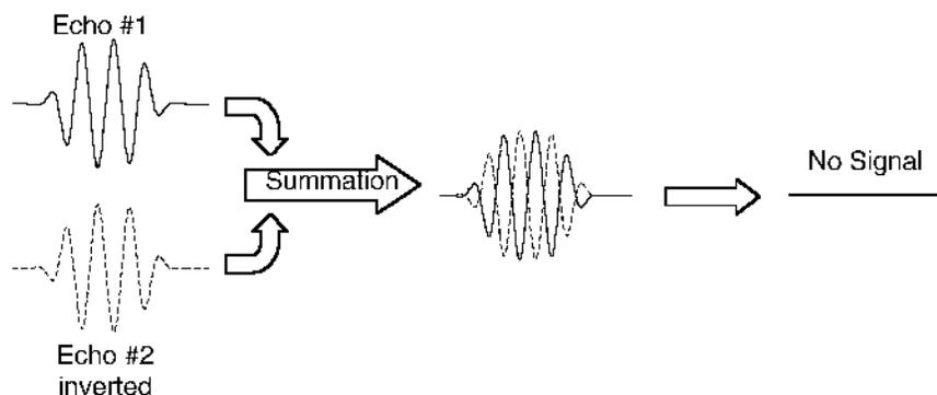
FIG. 2. By adding two consecutive bubble echoes from inverted pulses, pulse inversion cancels fundamental echoes without filtering.
