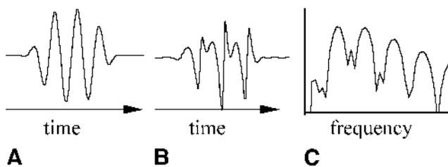
FIG. 1. A. Incident acoustic wave. B. Nonlinear bubble echoes. C. Frequency spectrum of bubble echoes.
