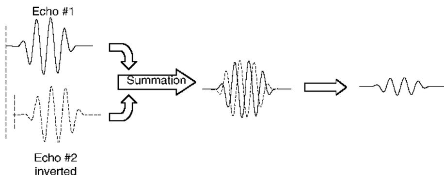
FIG. 5. Incomplete tissue echo cancellation with pulse inversion imaging resulting from motion between pulses.
