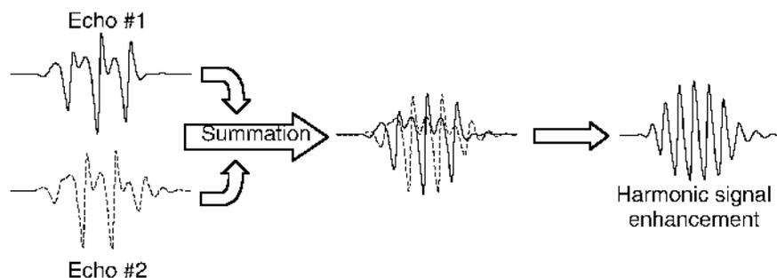
Any linear target that responds equally to positive and negative pressures will reflect back to the transducer equal but opposite echoes. These are then added in the beam former and all stationary linear targets cancel, as shown in Fig. 2.
