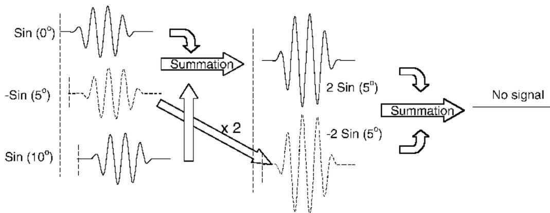
FIG. 6. Increased sensitivity and tissue motion cancellation with power pulse inversion imaging by summing multiple pulses.
