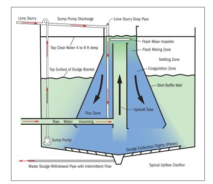
Schematic of sludge recycling process. We decided we needed to change our standard operating procedures if we wanted to bring the finished water turbidity down as low as reasonably possible and stay well within required standards, providing the very best finished water quality that we could.
