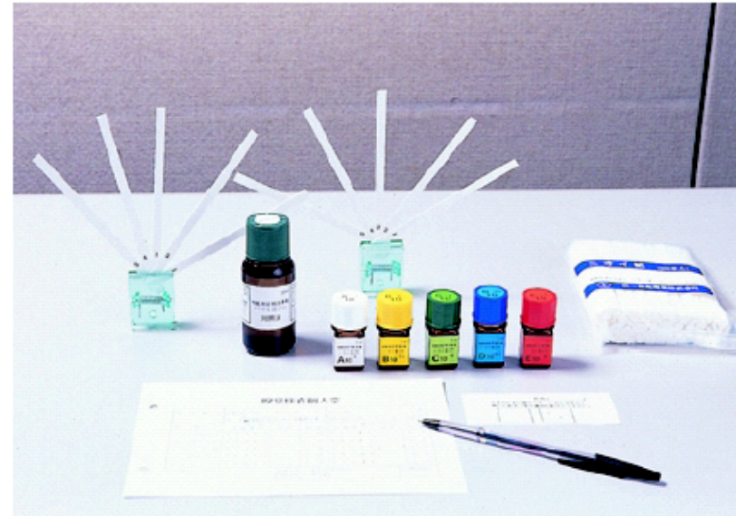
Standard Odorants for Aptitude Test: There are five standard odors used in the aptitude test including odor "smells like flowers" and odor "smells like sweaty socks."
